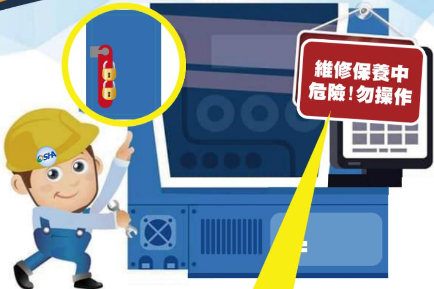
Under repair / maintenance ° Danger! Do not operate
